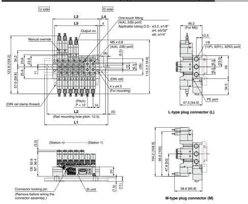
The dashed lines indicate the DIN rail mounting [-D].
