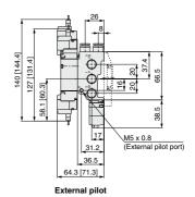
The dashed lines indicate the DIN rail mounting [-D].
