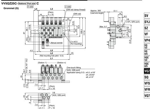
The dashed lines indicate the DIN rail mounting [-D]. 1/8
