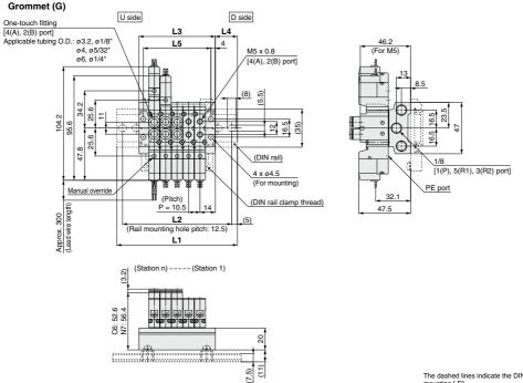
The dashed lines indicate the DIN rail mounting [-D].
