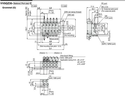
1/4 The dashed lines indicate the DIN rail mounting [-D].
