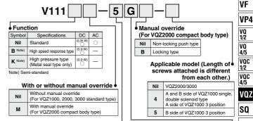
Coil voltage 100 VAC (50/60 Hz) 1 2 200 VAC (50/60 Hz) 110 VAC [115 VAC] (50/60 Hz) 3 4 220 VAC [230 VAC] (50/60 Hz) 5 24 VDC 12 VDC
