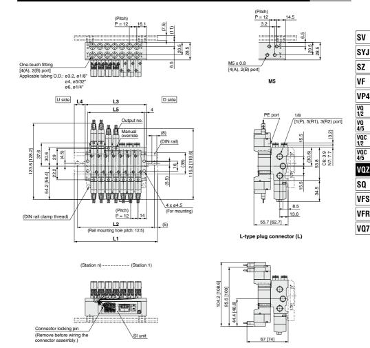
The dashed lines indicate the DIN rail mounting [-D]. Unless otherwise indicated, dimensions are the same as L-type plug connector (L). [ ]: AC
