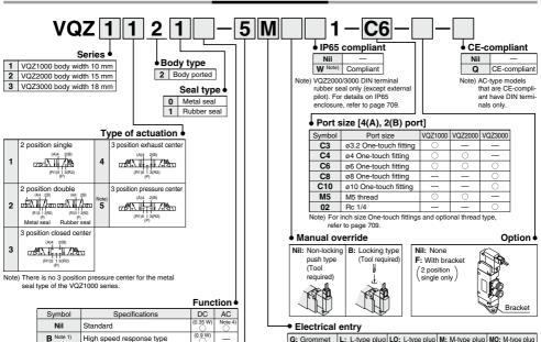
KR Note 1, 2, 3) High pressure/External pilot type (Metal seal type only)
