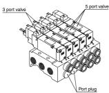
When port plug is used on 2 (B) port, indicate CM in manifold part no. and port size, and specify the port plug location by the manifold specification sheet.
