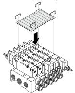
When shipping the manifold with the name plate attached, please order using the manifold option symbol [-N].
