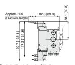
The dashed lines indicate the DIN rail mounting [-D].
