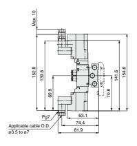
The dashed lines indicate the DIN rail mounting [-D].
