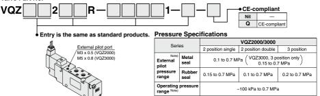
Note) In case of the high pressure type, upper limit of max. operating pressure and external nilot pressure range is 1 MPa
