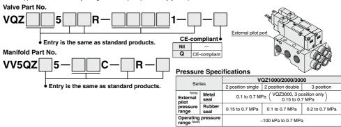
Note) In case of the high pressure type, upper limit of max. operating pressure and external pilot pressure range is 1 MPa.
