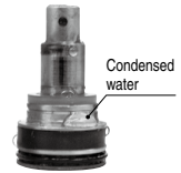
Grease deteriorates or is washed away.
