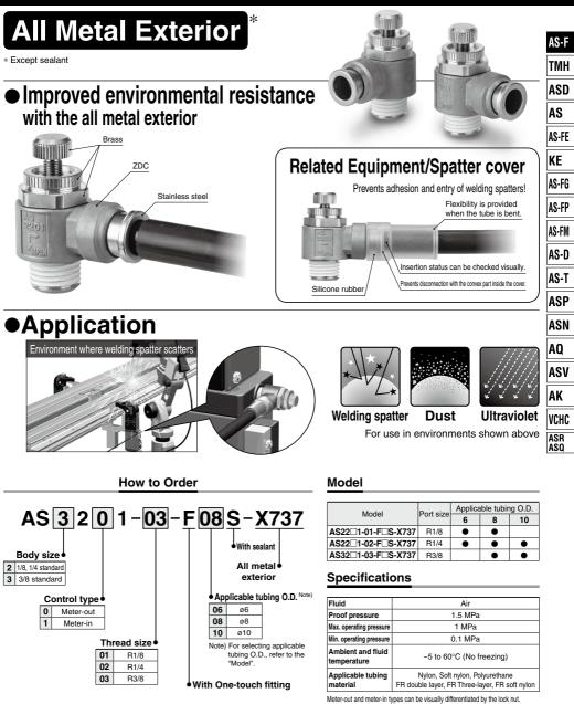
Meter-out and meter-in types can be visually differentiated by the lock nut. The lock nut on the meter-out type is brass color, while the meter-in type is black. 607
