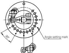
2. Then, make sure the angle is correct and fasten the screw to prevent an unintended change in angle.
