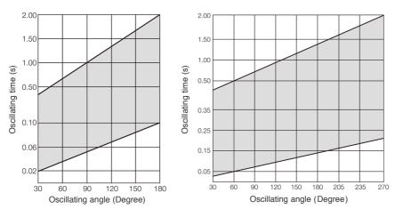
Note: Operate HI-ROTORs within the range of duration shown in above charts. Otherwise, the HI-ROTOR will tend to move in stick-slip motion.
