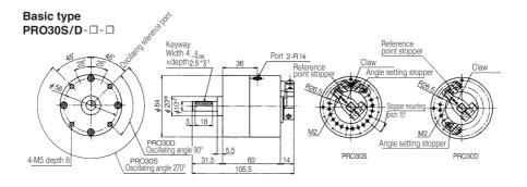
With foot plate PRO30S/D-□-□-L1 With flange plate PRO30S/D-□-□-P
