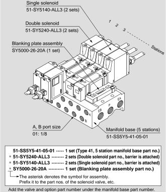
Add the valve and option part number under the manifold base part number. In the case of complex arrangement, specify them on the manifold specification sheet.
