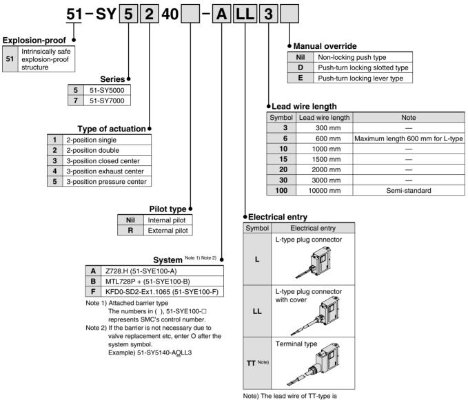
Note) The lead wire of TT-type is connected to the terminal block.
