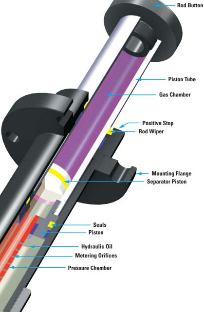
In the normal "ready" condition the piston rod is fully extended. When the impacting load strikes the buffer the hydraulic oil behind the piston is forced through a series of metering orifices. The number of metering orifices in action reduces proportionally through the stroke and the
