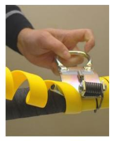
Start by rotaring the spiral 1-2 rounds onto the hose / hose bundle (if spiral is long it is better to start from the middle).
